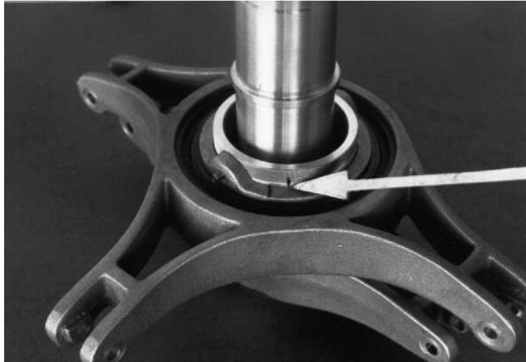
Photo 16: TIGHTEN SET SCREWS IN COLLAR.
